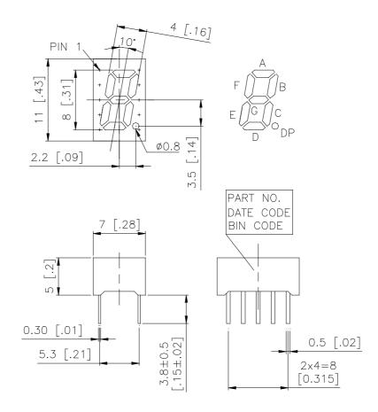
NOTES: 1.All dimensions are in millimeters. Tolerances are  $\pm$  0.25mm (0.01") unless otherwise noted. 2.Pin tip's shift tolerance is  $\pm$ 0.4mm.
