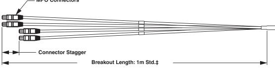
‡Breakout length tolerance is 12.7cm (+5")/-0
