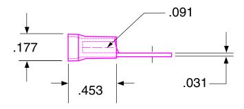
Max Electric Currrent: 16-14 AWG : 27 Amp Max Electric Rating: 75° C / 600 V Max
