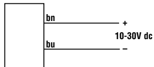
Emitters with Attached Cable
