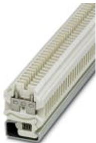
Feed-through terminal block, connection method: screw connection, cross section: 0.2 mm<sup>2</sup> - 4 mm<sup>2</sup>, 24 - 12 AWG, width: 6.2 mm, color: white, mounting type: NS 32, insulation material: ceramic
