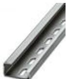
G-profile DIN rail, material: Steel, perforated, height 15 mm, width 32 mm, length 2 m
