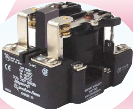
199B DPDT WITH MAGNETIC BLOWOUT FOR DC ARC QUENCHING 10 AMPS, 110 VDC
