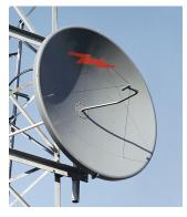
3.0 m | 10 ft Standard Parabolic Unshielded Antenna, dual-polarized, 10.200–10.700 GHz, CPR90G, gray antenna, with flash, standard pack—one-piece reflector
