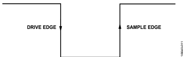
Figure 32. SPI Mode 3 SCLK Edges
