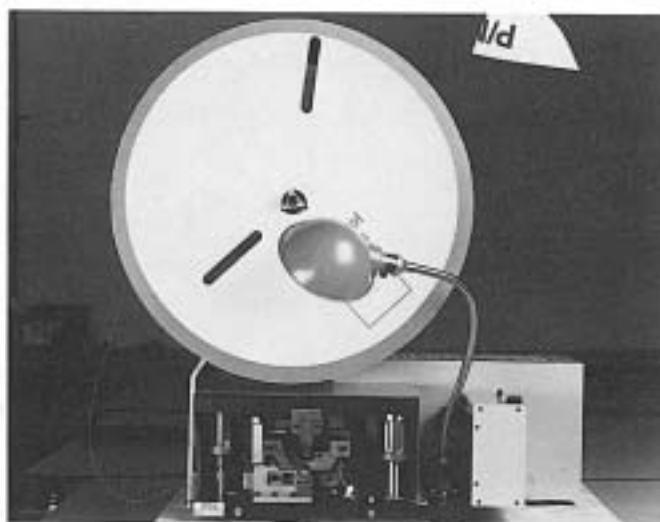
semi-automatic stripper/crimper machine 359-634 - strips and terminates discrete wire to open barrel, reel fed contacts. Used on stamped and formed 117 series contacts, auto-feed system maximizes production of crimp terminations of non-metallic insulated wire in ranges of #30-20 AWG. Termination rates can easily exceed 1500 wires per hour.
