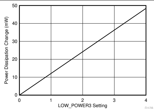
Figure 6-13. Power Dissipation Change vs LOW_POWER3 register setting
