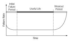
Life Cycle of an Aluminum Electrolytic Capacitor
