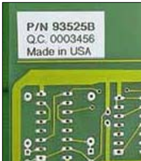
Circuit board labeling
