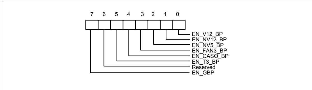
Bit 7 : Enable Global BEEP. Write 1, enable global BEEP output. Default 1. Write 0, disable all BEEP output.
