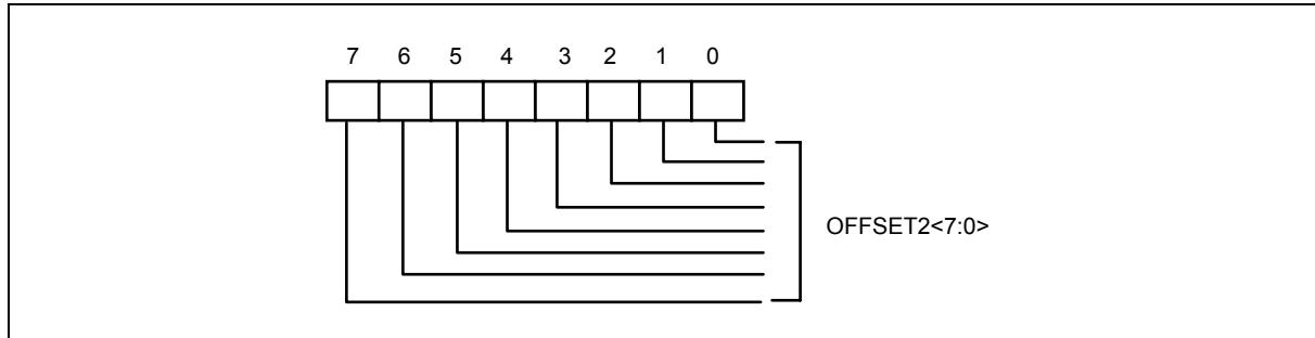
Bit 7-0 : Temperature 2 base temperature. The temperature is added by both monitor value and offset value.
