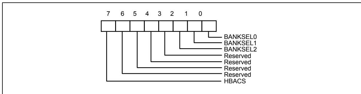
Bit 7 : HBACS- High byte access. Set to 1, access Register 4Fh high byte register. Set to 0, access Register 4Fh low byte register. Default 1.
