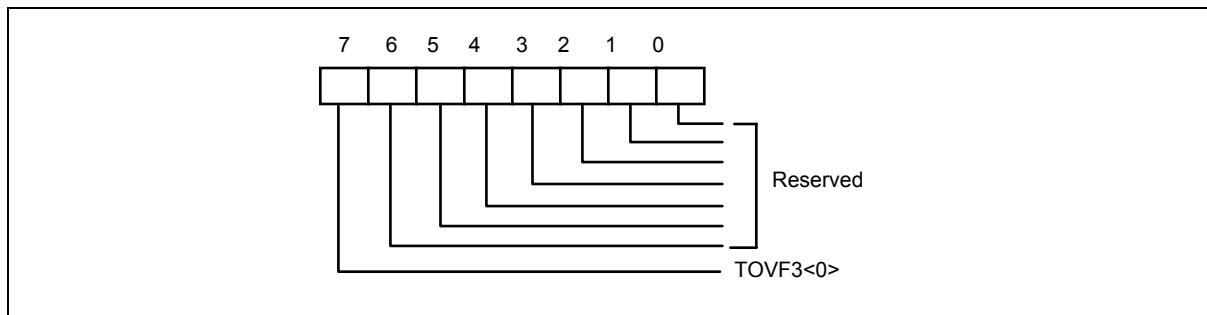
Bit 7 : Over-temperature bit 0, which is low Byte.
