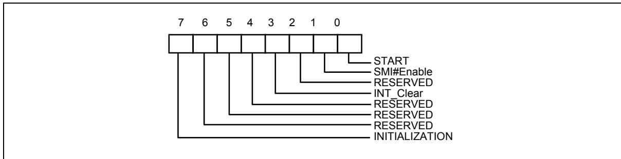
Bit 7 : A one restores power on default value to all registers except the Serial Bus Address register.
