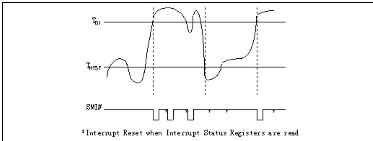
Figure. 8.10 Temperature 2, 3 SMI# Comparator Interrupt Mode
