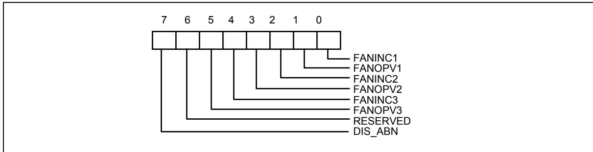
Bit 7 : Disable power-on abnormal the monitor voltage including V-Core A and +3.3V. If these voltage exceed the limit value, the pin (Open Drain) of BEEP will drives 300Hz and 600Hz frequency signal. Write 1, the frequency will be disabled. Default is 0. After power on, the system should set 1 to this bit to 1 in order to disable BEEP.
