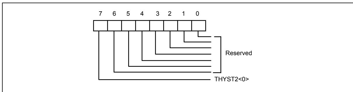
Bit 7 : Hysteresis temperature bit 0, which is low Byte.
