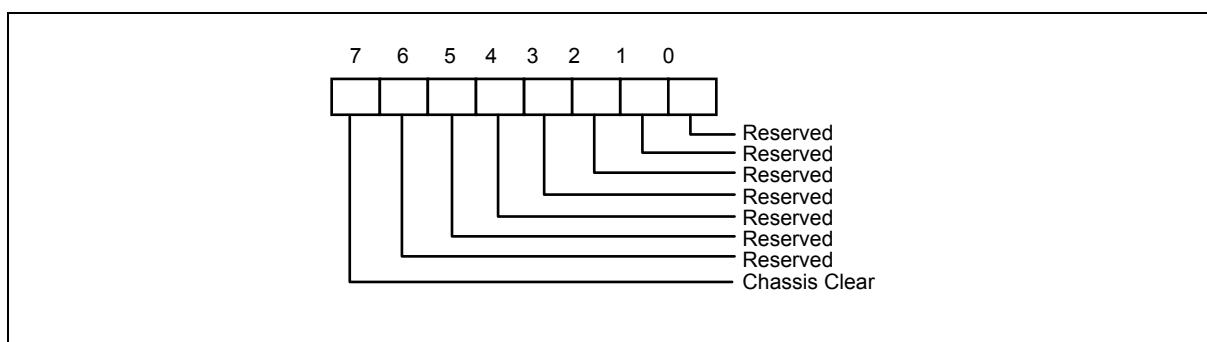
Bit 7 : **Clear Chassis Intrusion Event.** Write “1” will make Hardware Monitor Register Index 42, bit 4 cleared to “0” . This bit self clears after clearing Chassis Intrusion event. For W83627HF A Version, Clear Chassis Intrusion Event has been changed from this bit to LDA CRE6[6].
