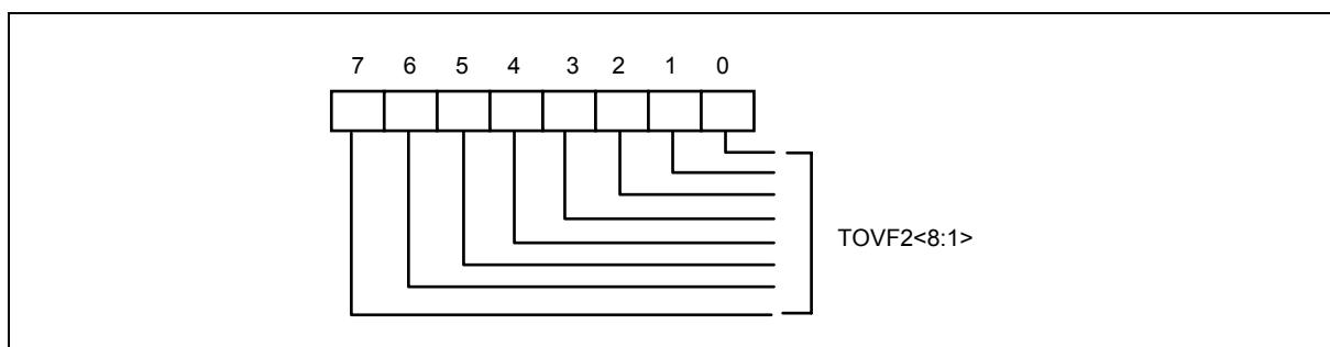
Bit 7-0 : Over-temperature bit 8-1, which is High Byte. The temperature default 80 degree C.
