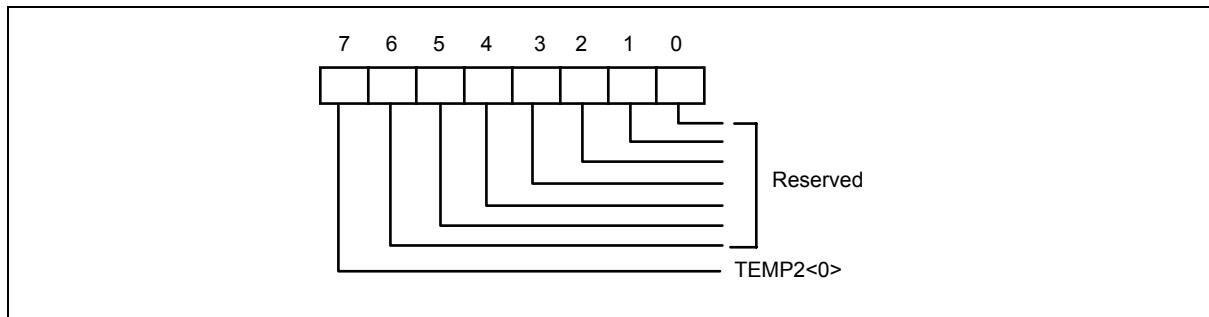
Bit 7 : Temperature <0> of sensor2, which is low byte.
