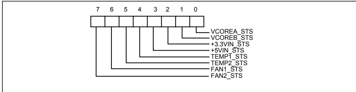
Bit 7 : FAN 2 Status. Set 1, the fan speed counter is over the limit value. Set 0, the fan speed counter is in the limit range.
