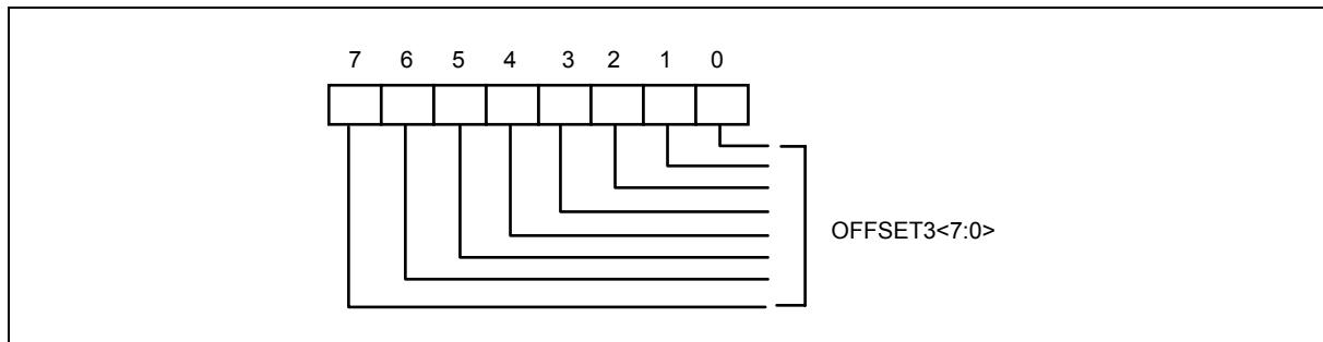
Bit 7-0 : Temperature 3 base temperature. The temperature is added by both monitor value and offset value.
