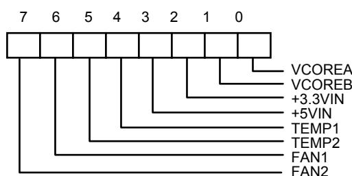
Bit 7-0 : A one disables the corresponding interrupt status bit for SMI interrupt.
