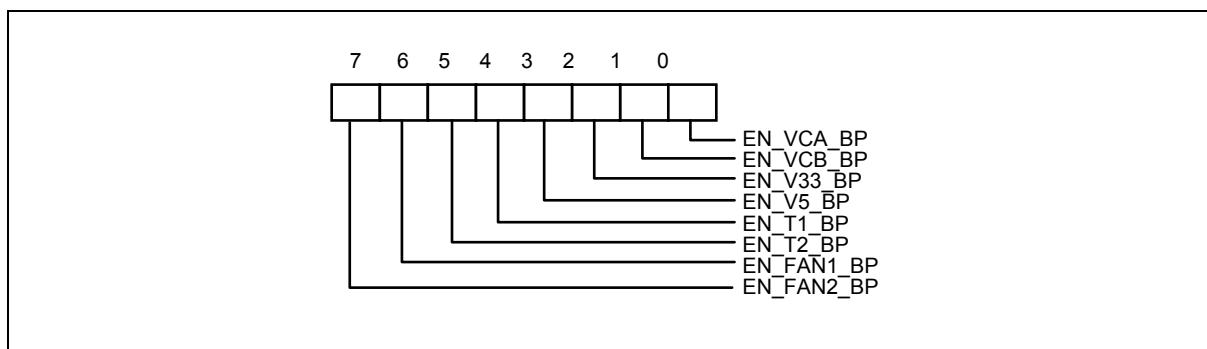
Bit 7 : Enable BEEP Output from FAN 2 if the monitor value exceed the limit value. Write 1, enable BEEP output, which is default value.
