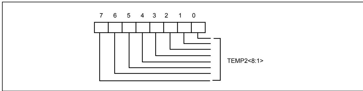
Bit 7 : Temperature <8 : 1> of sensor 2, which is high byte.
