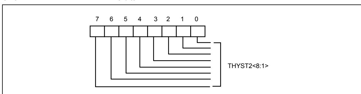
Bit 7-0 : Temperature hysteresis bit 8-1, which is High Byte. The temperature default 75 degree C.
