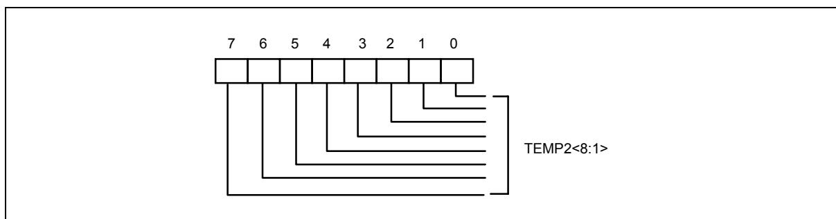
Bit 7-0 : Temperature <8 : 1> of sensor 2, which is high byte.
