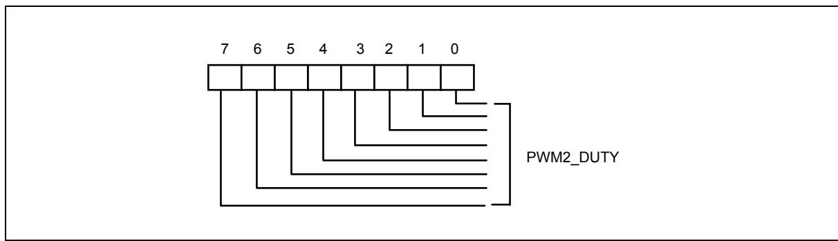
Bit 7 : PWMOUT2 duty cycle control. Write FF, Duty cycle is 100%, Write 00, Duty cycle is 0%.
