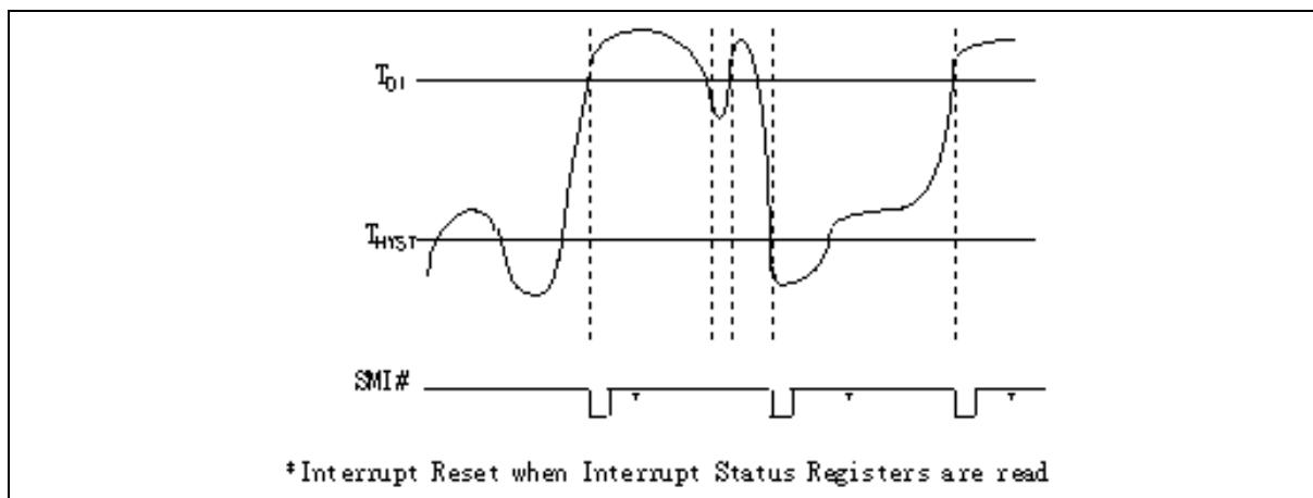
Figure. 8.11 Temperature 2, 3 SMI# Two-Times Interrupt Mode
