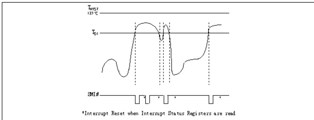
Figure. 8.8 Temperature 1 SMI# Comparator Interrupt Mode
