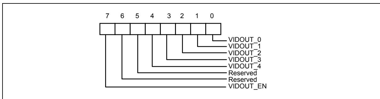
Bit 7 : VID Output Enable. Set 1, enable VID pins to output. Set 0, disable VID pins to output. Default is 0.
