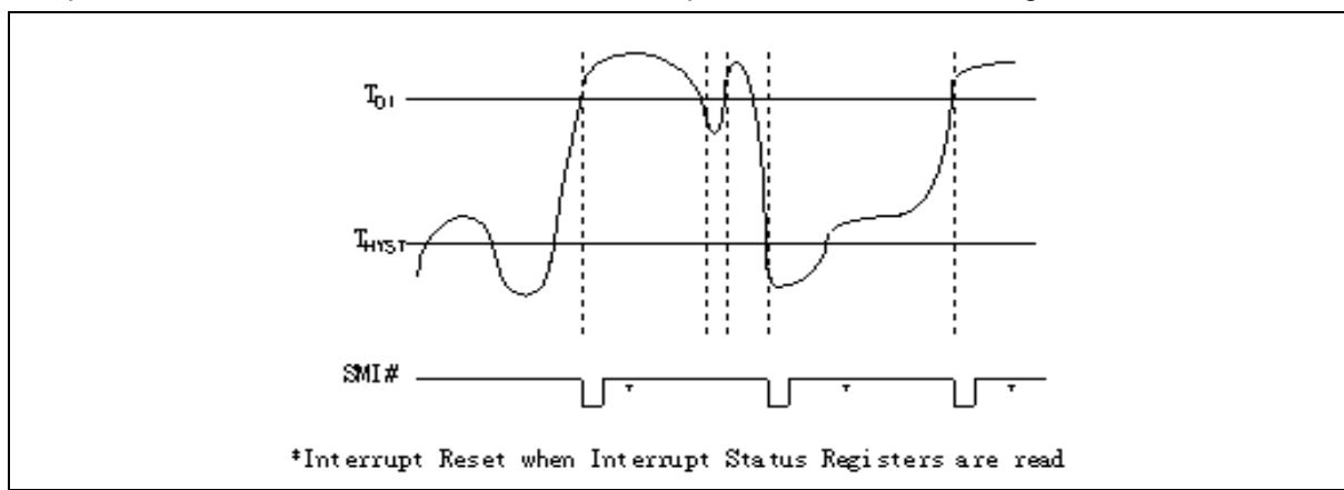
Figure. 8.9 Temperature 1 SMI# Two-Times Interrupt Mode
