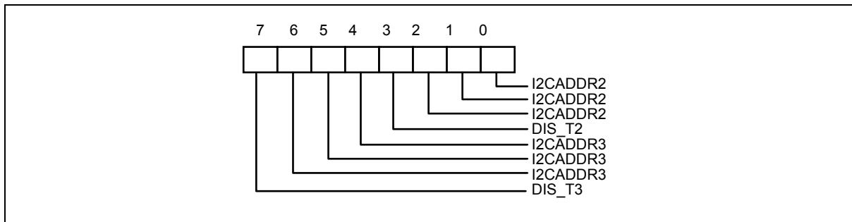
Bit 7 : Set to 1, disable temperature sensor 3 and can not access any data from Temperature Sensor 3.
