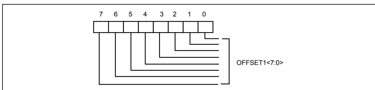
Bit 7-0 : Temperature 1 base temperature. The temperature is added by both monitor value and offset value.
