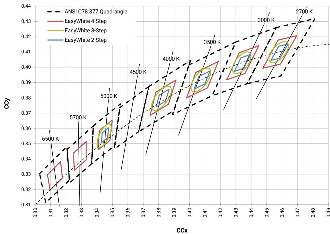
CREE ANSI WHITE BINS PLOTTED ON THE 1931 CIE COLOR SPACE ( $T_J = 85^\circ\text{C}$ )
