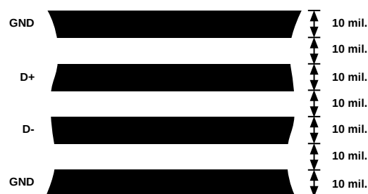
Figure 14. Arrangement of Signal Tracks
