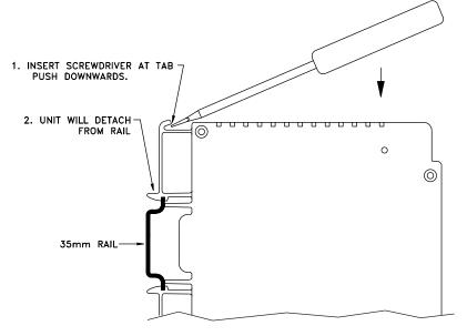
Figure 2.3 Removal - DIN Rail iServer
