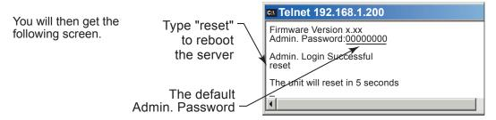
Figure 3.3 Telnet Login into the iServer
