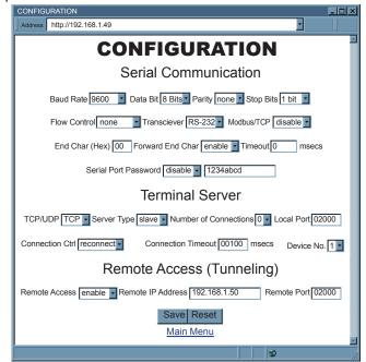
Figure 4.16 shows the valid values that need to be set in the Local iServer. The Baud Rate, Data Bits, Parity, Stop Bits, Flow Control, and Transceiver values depend on what the attached device to the iServer supports.
