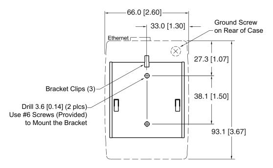
Figure 2.1 Mounting - Wall Mount iServer
