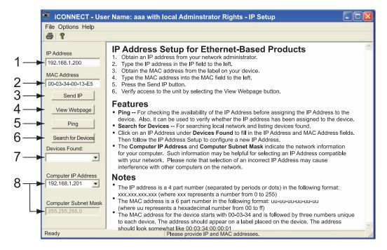
Figure 4.2 Assigning an IP Address using iConnect
