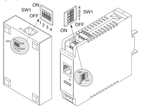
Figure 2.4a DIP Switch Wall Mount iServer
