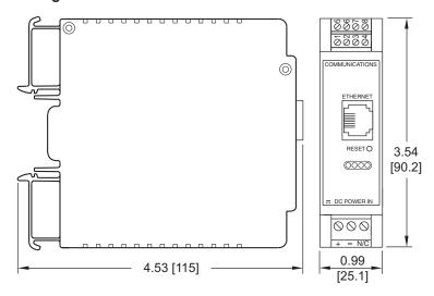
Figure 5.2 DIN Rail iServer Dimensions
