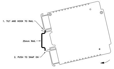
Figure 2.2 Mounting - DIN Rail iServer
