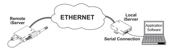
Figure 4.14 PC-to-Device Communication
