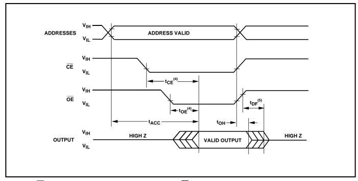
**NOTE:** 4.  $\overline{\text{OE}}$  may be delayed up to  $t_{\text{CE}} - t_{\text{OE}}$  after the falling edge of  $\overline{\text{CE}}$  without impact on  $t_{\text{CE}}$ .
