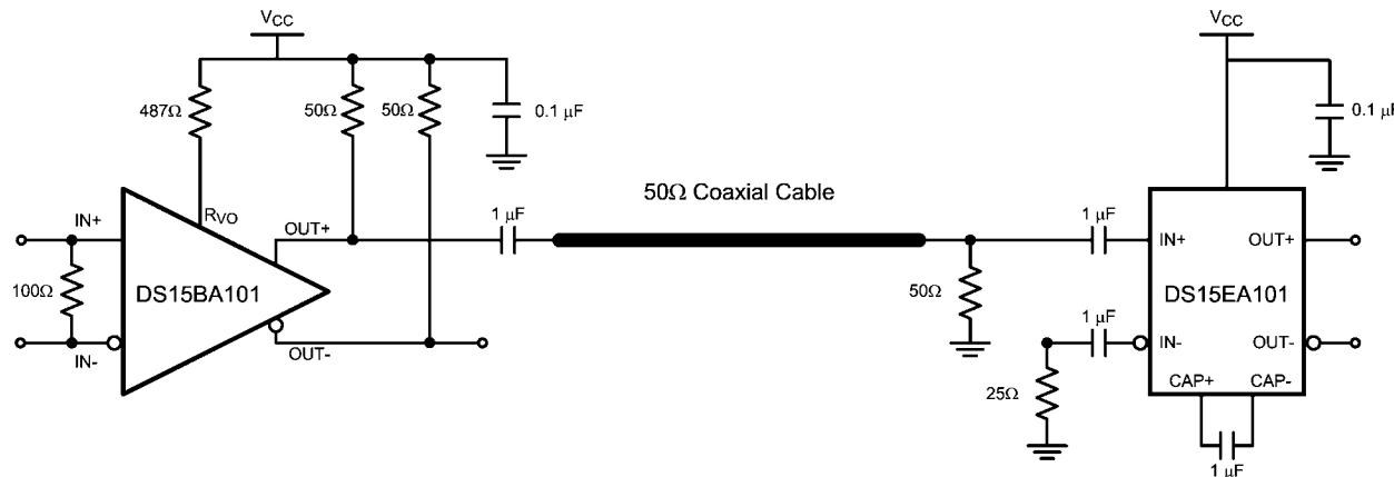
Cable Extender Chipset Connection Diagram for  $50\Omega$  Coaxial Cables
