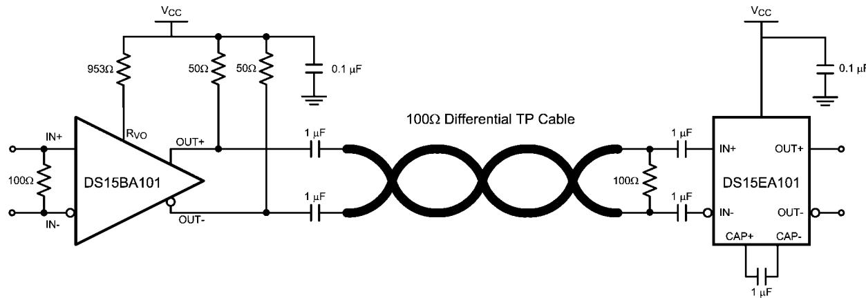
Cable Extender Chipset Connection Diagram for  $100\Omega$  Differential Cables
