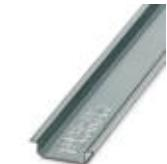
DIN rail, unperforated, Standard profile, width: 35 mm, height: 7.5 mm, acc. to EN 60715, material: Steel, Galvanized, white passivated, length: 2000 mm, color: silver
