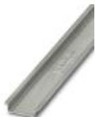
DIN rail, unperforated, Standard profile, width: 35 mm, height: 7.5 mm, acc. to EN 60715, material: Steel, galvanized, passivated with a thick layer, length: 2000 mm, color: silver
