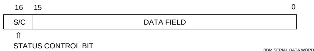
Figure 3-11 BDM Serial Data Word
