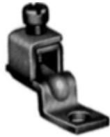
**Lug-It®** connectors are designed to grip the cable firmly between the strong body and the serrated copper tongue. Double laps at the top give greater thread strength and lock the screw when it is tight. The copper tongue makes a low resistance terminal.
