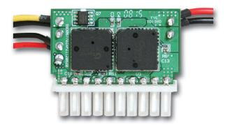
GADIWA-1120 is a DC-DC converter for socket type. It normally support 96Watts and maximum can reach to 120Watts. GADIWA-1120 socket type design can save more space and cost, it's not only capability for fan-less system but also suitability for different application. Besides, the converter is made and tested by automatic production line; therefore, it can provide high quality and performance.
