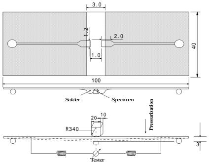
NOTE) \*1 The shaded area shows the solder resist treatment.
