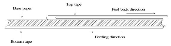
4.2 Base tape should not adhere to top tape when top tape is peeled back, and peel back direction is as follows.
