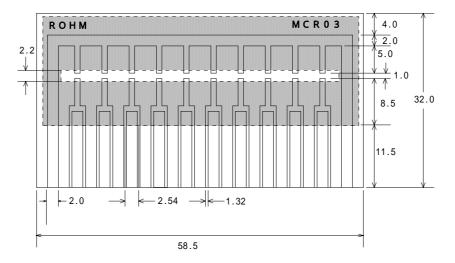
NOTE) \*1 The shaded area shows the solder resist treatment.
