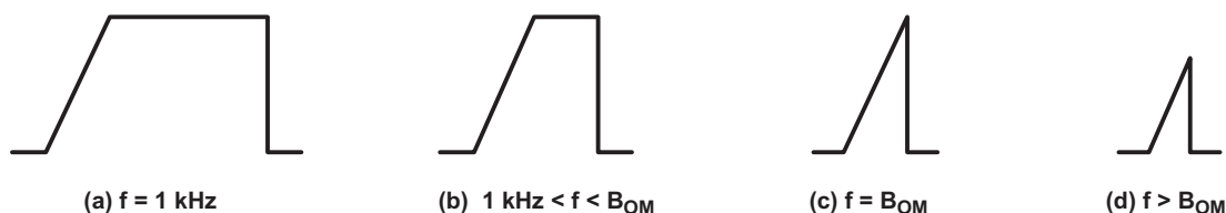
Figure 5. Full-Power-Response Output Signal
