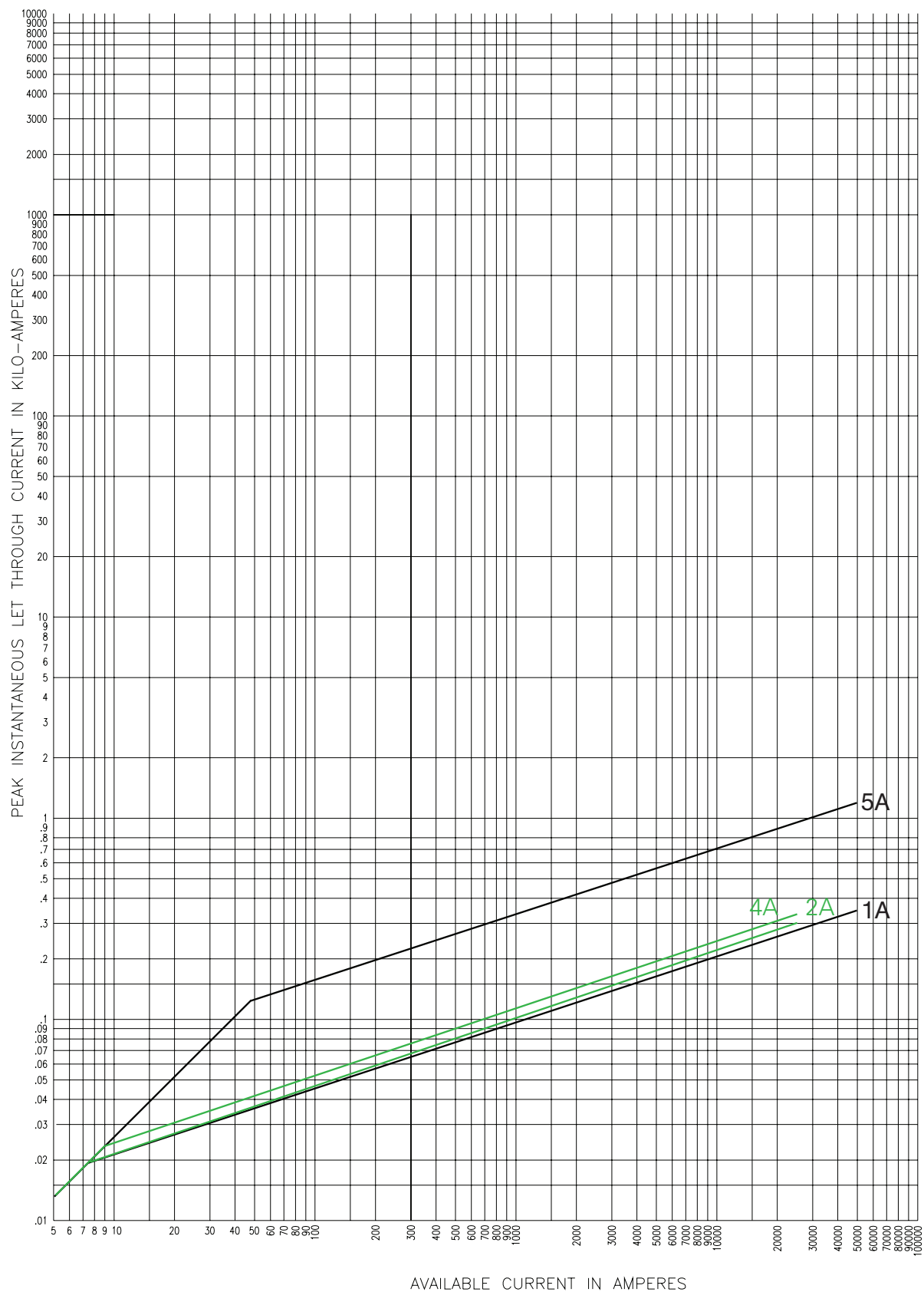
8.3kV Peak let-through curves for 8NCLPT_
