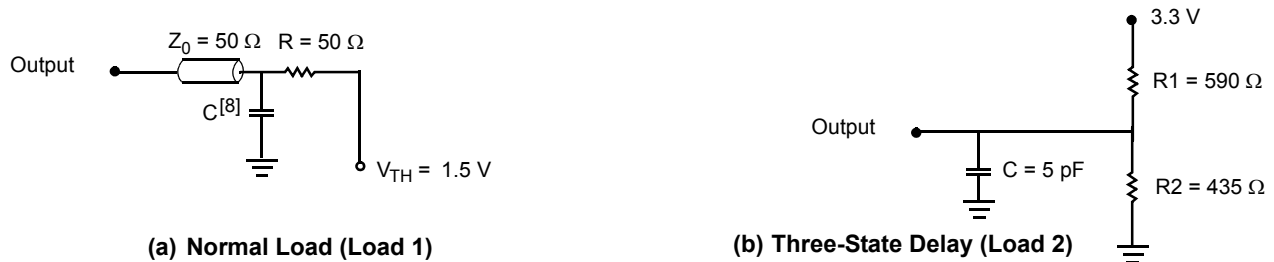
Figure 3. AC Test Load and Waveforms
