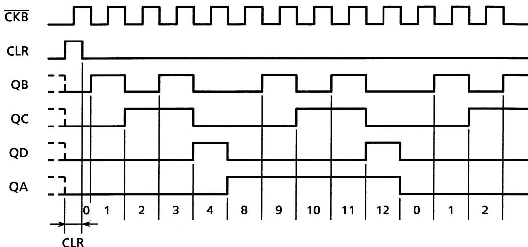
Note: QD connected to  $\overline{\text{CKA}}$
