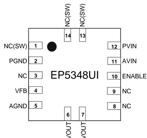
Figure 2: EP5348UI Pin Out Diagram (Top View)
