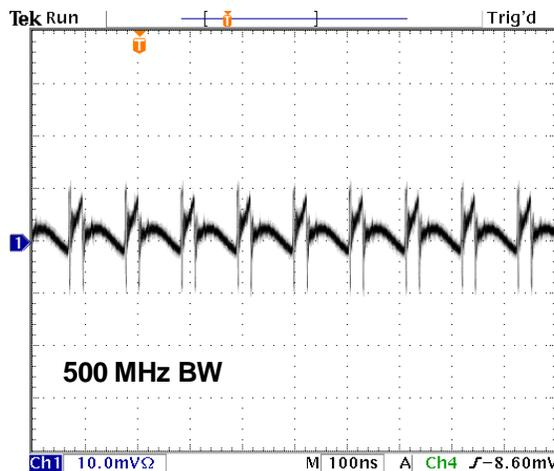
Output Ripple:  $V_{IN} = 5V$ ,  $V_{OUT} = 1.0V$ ,  $I_{out} = 400mA$
