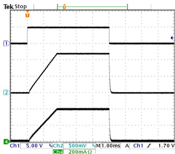
**Power Up/Down into 3Ω load:  $V_{IN}/V_{OUT} = 5.5V/3.3V$ ,**
