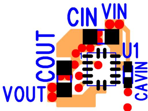
Figure 4: Top PCB Layer Critical Components and Copper for Minimum Footprint
