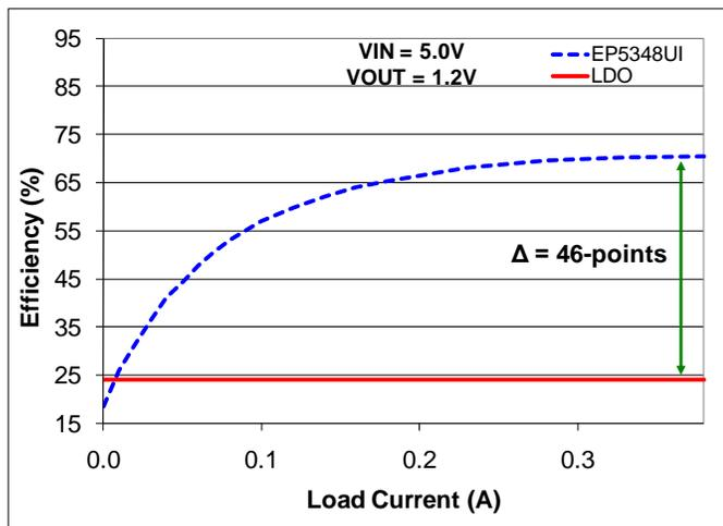
Integrated magnetics enables a tiny solution footprint, low output ripple, and high reliability, while maintaining high efficiency. The complete solution size is similar to an LDO and much smaller than a comparable DCDC.
