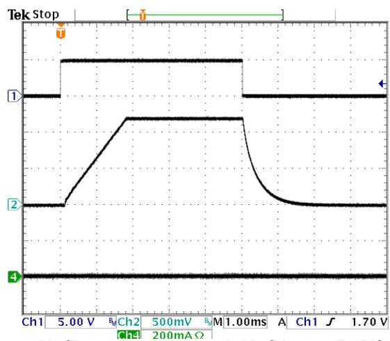
**Power Up/Down at No Load:  $V_{IN}/V_{OUT} = 5.0V/1.2V$ ,**
