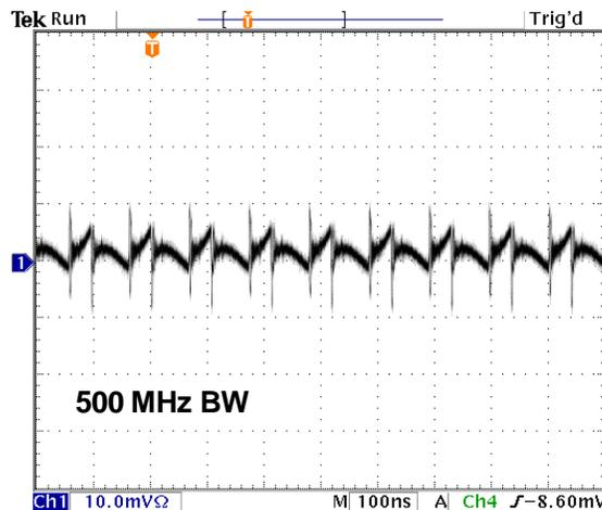
Output Ripple:  $V_{IN} = 3.3V$ ,  $V_{OUT} = 1.0V$ ,  $I_{out} = 400mA$
