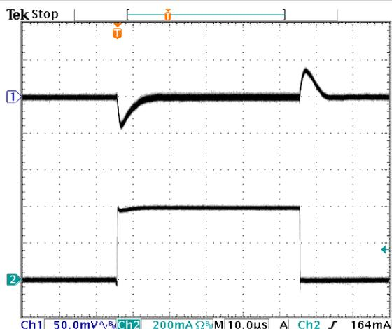
**Load Transient:  $V_{IN} = 5V$ ,  $V_{OUT} = 1.0V$**
