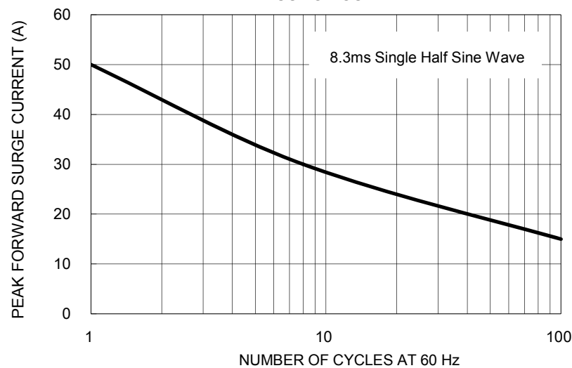
FIG. 3 MAXIMUM NON-REPETITIVE PEAK FORWARD SURGE CURRENT
