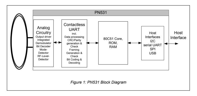
The Analog circuitry handles the modulation and demodulation of the analog signals according to the card mode, reader /writer mode and NFC mode communication scheme.
