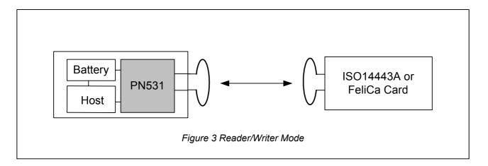
In the reader/ writer mode the PN531 enables communication to a passive ISO14443A/MIFARE® or FeliCa<sup>TM</sup> card
