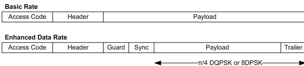
Basic Rate and Enhanced Data Rate Packet Structure
