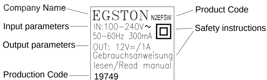
Figure 7 Example of Label on plastic housing by laser marking
