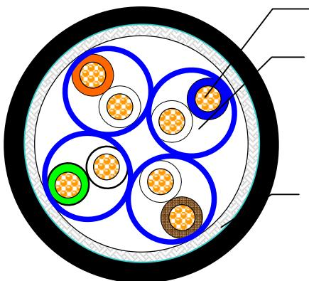
Conductor (26AWG/7 – 7x0.16mm Stranded Copper)
