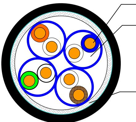
Conductor (23AWG/1 – Solid Bare Copper)
