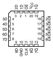
To ensure the high-impedance state during power up or power down,  $\overline{OE}$  should be tied to  $V_{CC}$  through a pullup resistor; the minimum value of the resistor is determined by the current-sinking capability of the driver.
