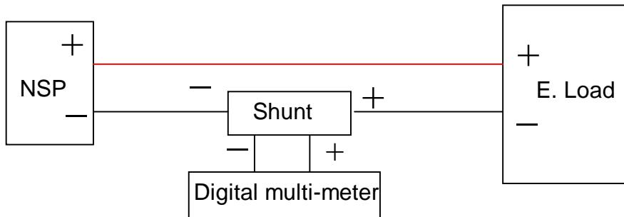
2. Press and hold the current control knob and then turn ON the NSP power switch, release the voltage control knob once LCD display turns on. Now the unit is under calibration mode.
