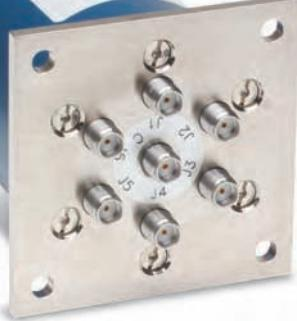
The CR-39 Switch is a broadband, multi-throw, electromechanical coaxial switch designed to switch a microwave signal from a common input to any of 3, 4, 5, or 6 outputs. The characteristic impedance is 50 Ohms. The switches are small using the popular connector spacing on a 1.062" dia. circle. Each position has an individual actuator mechanism allowing random position selection. This also minimizes switching time.
