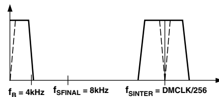
d. Final Filter LPF (HPF) Transfer Function
