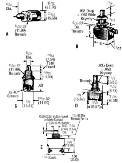
**Multi-Purpose AC/DC Pushbutton Switches**
