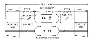
Coating Diameter (max): 0.5A-3.0A: 2.80mm 5.0A: 2.90mm
