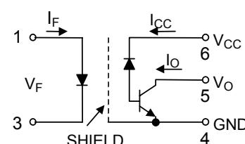
A 0.1- $\mu\text{F}$  bypass capacitor must be connected between pins 4 and 6.
