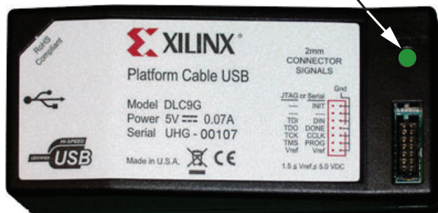
Figure 11: Status LEDs Indicating Target Voltage
