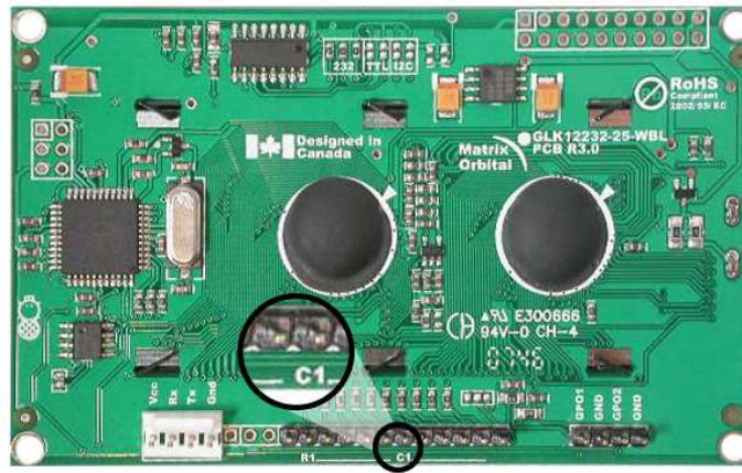
Figure 17: Manual Override Jumper
