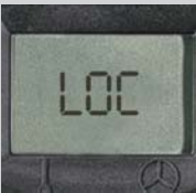
LOC Lockable Override Control
