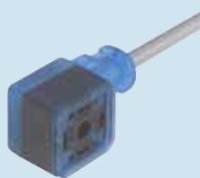
Cable socket with integrally molded lead (2 m), function indicator (LED) for pressure switch, gasket (captive) and central screw M3 (stainless steel, Phillips cross-head)
