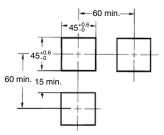
Note: 1. The mounting panel thickness should be 1 to 5 mm.
