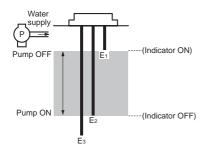
The pump stops when the water level reaches  $E_1$  (indicator ON) and starts when the water level drops below  $E_2$  (indicator OFF).
