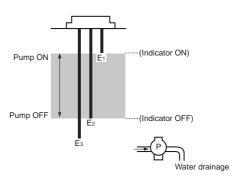
The pump starts when the water level reaches  $E_1$  (indicator ON) and stops when the water level drops below  $E_2$  (indicator OFF).
