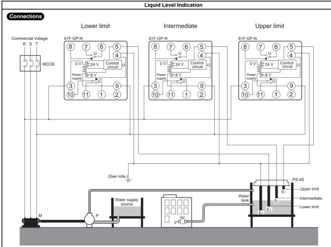
Note: The power supply phases (terminals 3 to 9) can be matched to use the same ground for the common Electrode (the longest Electrode, terminal 4).
