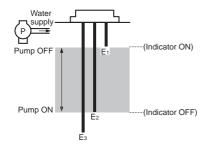
The pump stops when the water level reaches E<sub>1</sub> (indicator ON) and starts when the water level drops below E2 (indicator OFF).
