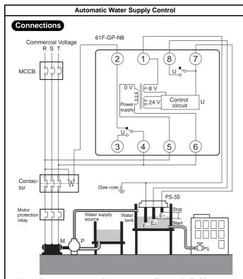
Note: Be sure to ground the common Electrode E<sub>3</sub> (the longest Electrode).
