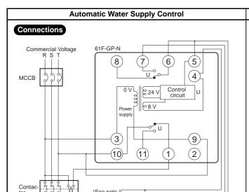
Note: Be sure to ground the common Electrode E<sub>3</sub> (the longest Electrode).
