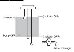
The pump starts when the water level reaches E<sub>1</sub> (indicator ON) and stops when the water level drops below E<sub>2</sub> (indicator OFF).
