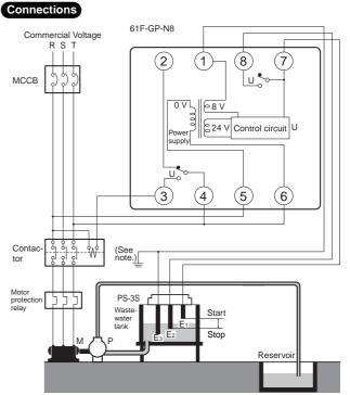
Note: Be sure to ground the common Electrode E<sub>3</sub> (the longest Electrode).
