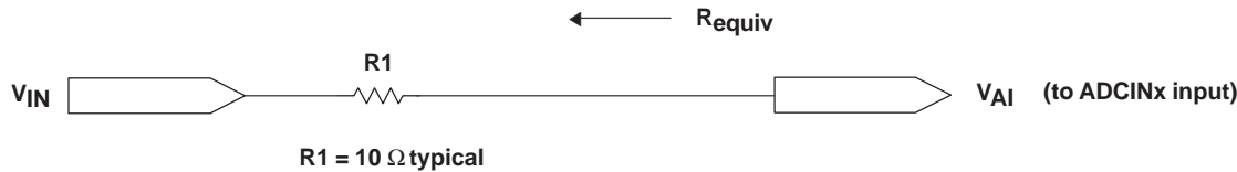
Figure 31. Typical ADC Input Pin Circuit
