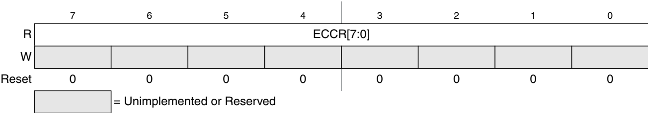
Figure 29-21. Flash ECC Error Results Low Register (FECCRLO)
