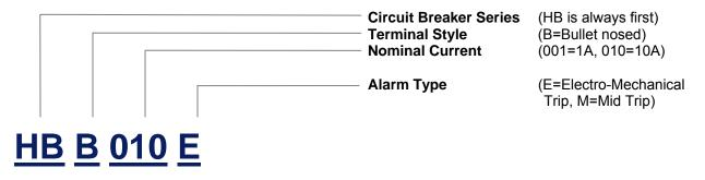
Plug in circuit breakers with bullet nosed terminals are available as follows. E trip breakers have black handles. M trip breakers have white handles.
