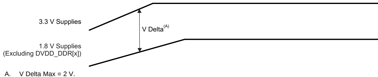
Figure 7-2. 3.3 V Supplies Rising Before 1.8 V Supplies Delta
